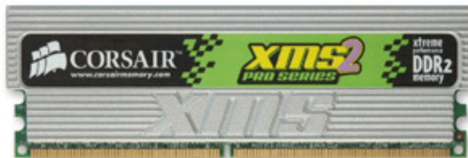
A DDR2 module with large heatspreaders *
